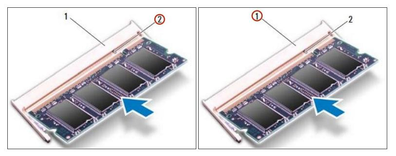
• Align the notch on the **NEW** memory module with the tab in the memory module connector.
