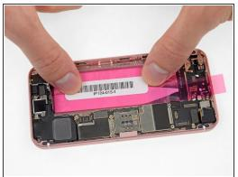
Press down on each strip to fully adhere it to the rear case, starting from the middle and working outward towards each end.
