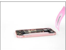
Peel away the large pink film liner and remove it completely.
