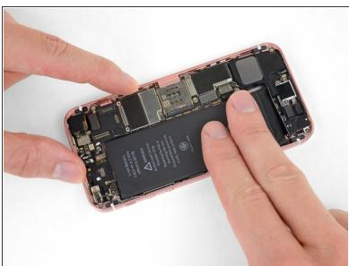
Press the battery firmly into place.
