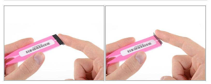
With the exposed adhesive facing down, fold the black tab up at a 90° angle.
