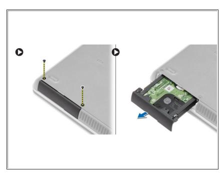
Remove the screws that secure the hard drive to the computer. Slide the hard drive out of the computer.
