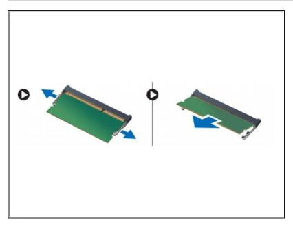
Pry the securing clips away from the memory module until it pops-up. Remove the memory module from its connector on the system board.
