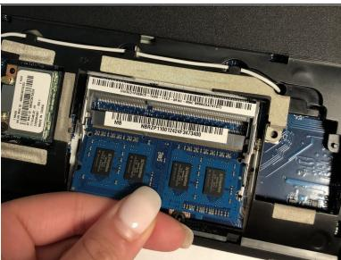
After removing the screw, push the tabs on the sides of the cards out. This will allow the RAM card
