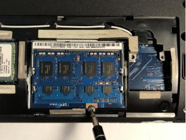
Remove the screw that is securing the RAM chip in place
