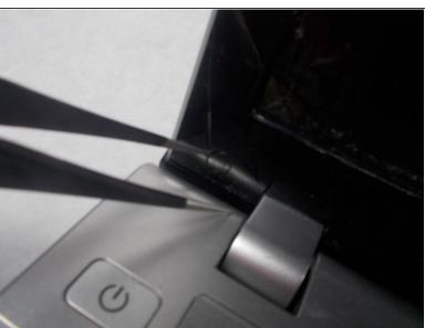
Use a pair of tweezers to carefully remove the two small pieces of plastic at the bottom of the screen.
