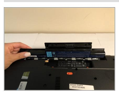
While holding the lever to the right, use your fingers to lift the battery up and out of the compartment.
