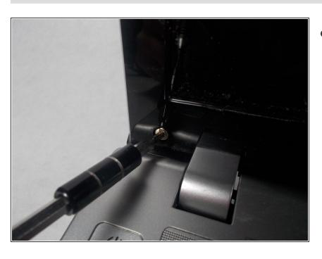
Use a Phillips #0 screwdriver to remove both screws.
