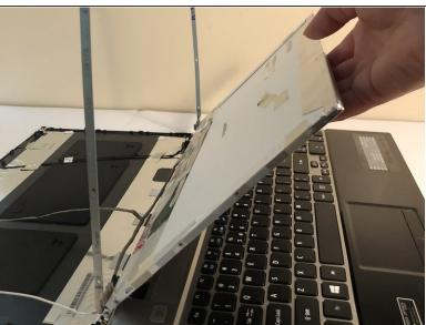
Use the Phillips #0 screwdriver to remove the three screws on each side of the screen.
