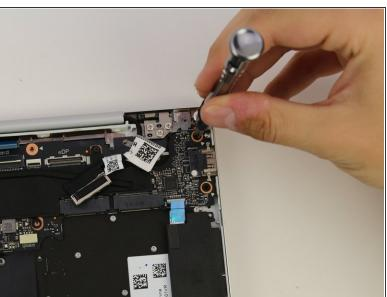
Remove the seven black 2mm screws using a PH1 screwdriver.
