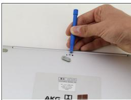
• Insert the plastic opening tool underneath the top-middle rubber covering and lift upwards to reveal the hidden screw.
