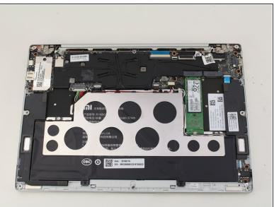
Remove the back of the laptop by gently lifting the casing upwards.
