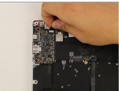
Remove the webcam connector by gently pulling the cable out by hand.
