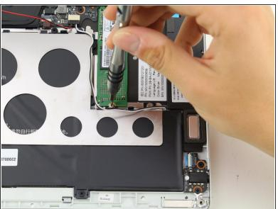
Remove the 1.5mm screw using the JIS #00 screwdriver.
