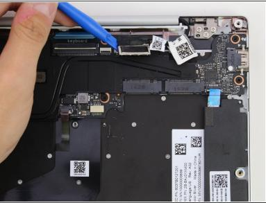
Lift the video cable on the connector using the plastic opening tool to disconnect it.
