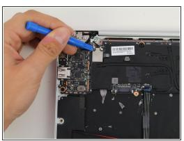
Disconnect the gray and black wire connectors using the plastic opening tool to lift them up.
