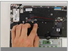
Remove the four ribbon cables by lifting the connector up with the plastic opening tool and pulling the ribbon cable out.
