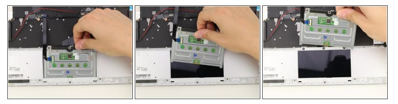
Lift the top end of the trackpad at a small angle and pull the trackpad out.
