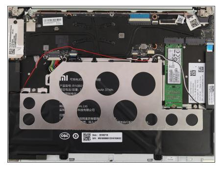
Detach the red wire from the tabs on the perimeter of the metal bracket.
