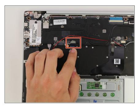
Gently remove the cable by pulling it out from the connector.
