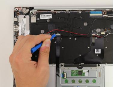
• Disconnect the trackpad cable from the motherboard by inserting the plastic opening tool under the white tab of the connector and pry up the white tab.
