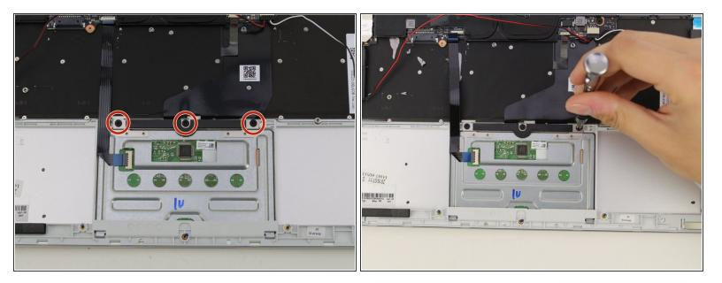
• Use a PH1 screwdriver to remove the three 2 mm screws.
