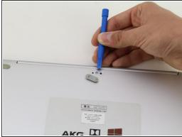
• Insert the plastic opening tool underneath the top-middle rubber covering and lift upwards to reveal the hidden screw.
