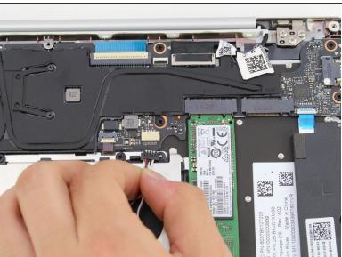
Gently pull the speaker connector out from the connection point using your hand.
