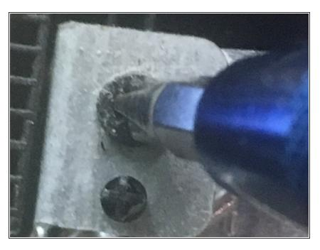
Remove the 2 screws from the top of the frame, One on each side.
