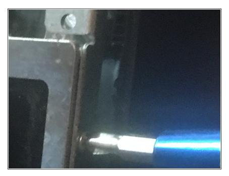
Remove the 4 screws holding the LCD to the frame. 2 on each side.
