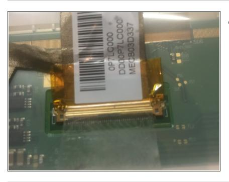
Lay the LCD down on the keyboard and remove the webcam cable (if you have one) and remove the video cable.
