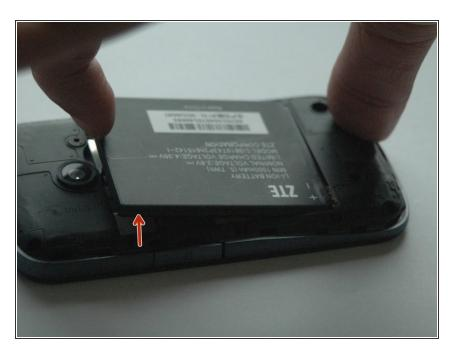
Remove the battery by inserting your fingernail at the top of the battery and lift it up.
