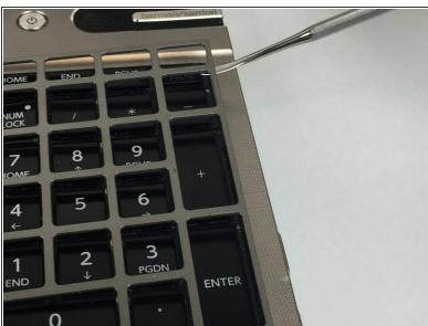
Use a plastic opening tool to pry up the keyboard cover.
