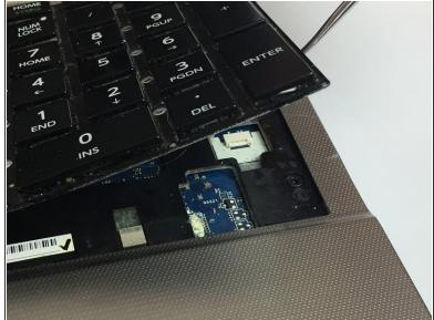
Use a plastic opening tool to pry up the keyboard.
