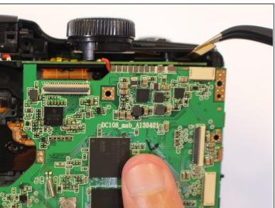
Using the tweezers, disconnect the orange cable connection at the top of the motherboard near the mode dial.
