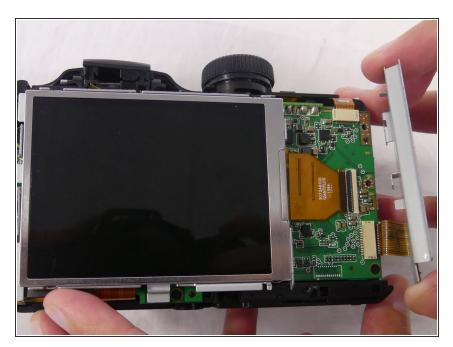
Pull the small metal switch plate to the side.
