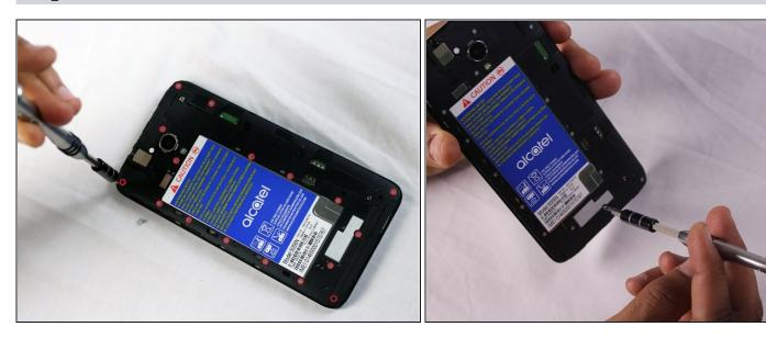
• Remove the seventeen Phillips #000 screws from the mid-frame.
