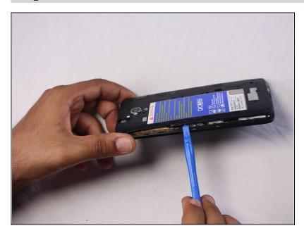
Pry off the mid-frame using a plastic opening tool, working your way around the perimeter.
