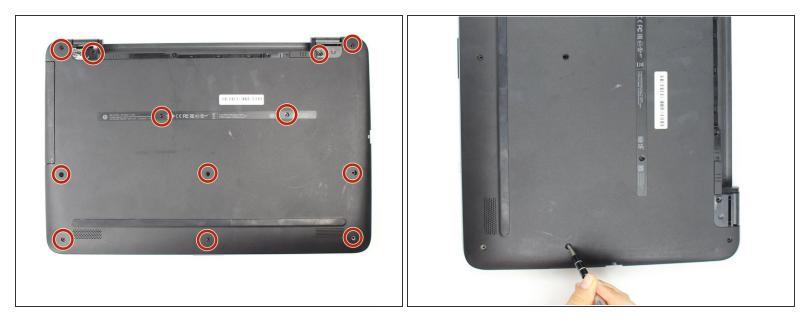
Turn off your computer before starting, and remove the battery.
