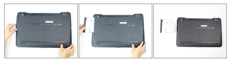
• Remove the optical drive by pushing it in and then it will pop out.
