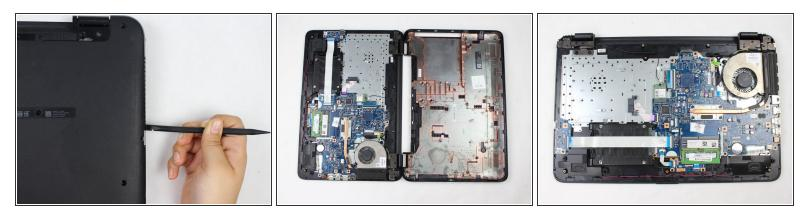
• Use a spudger to remove the back panel.
