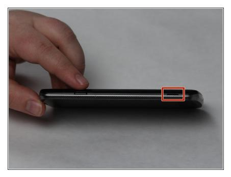
Place the plastic opening tool into the indent on the side of the phone and lift the back off the device.
