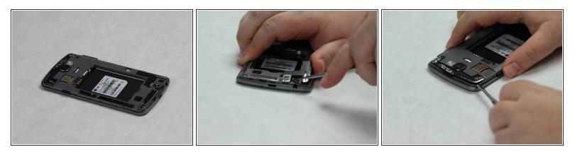
• Insert the spudger into the small groove under one of the two black pieces.
