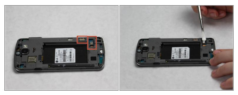
Using either your finger or the spudger, gently lift the metal clasps until they are no longer connected to the back of the phone.
