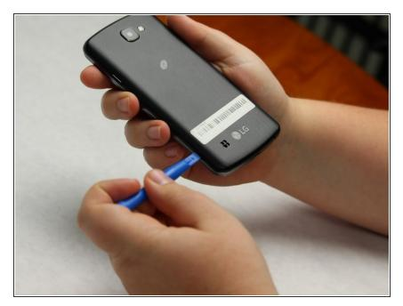
• Put the plastic opening tool in at a downward angle and push it up so that the back pops off.
