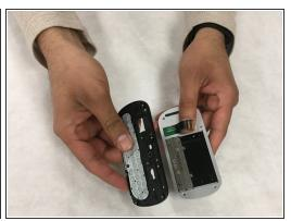
• There are six 2mm screws that connect the keypad piece to the other side of the phone. Using a Phillips #000 screwdriver, remove those screws and separate the two sides of the phone.
