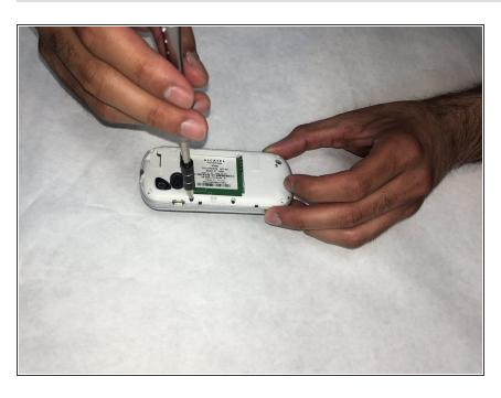
There are eight 2mm screws that must be removed from the back of the device using a Phillips #000 screwdriver. As you remove them it is wise to organize them into a small container or place them on a magnetic project mat for safe keeping.
