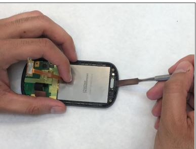
Voila! You now have access to the speaker. The face of the speaker is lightly adhered to the plastic case. Use the spudger to gently lift it from the plastic casing.
