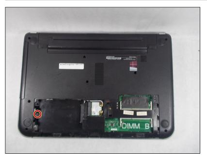
Now, remove the single screw that is securing the hard drive to the laptop noted by the red circle.
