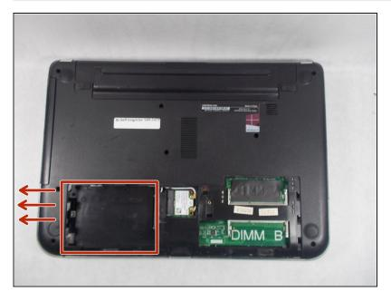
Now carefully lift then pull the hard drive out to the left until it detaches
