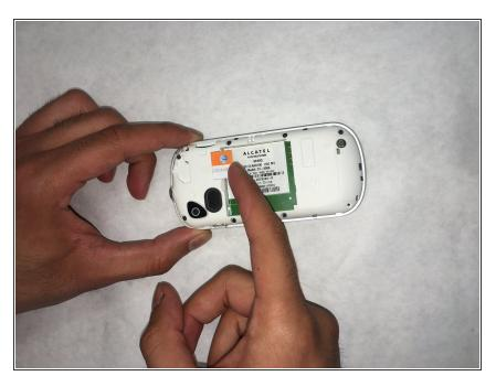
Once the battery has been removed the SIM card is easily accessible.
