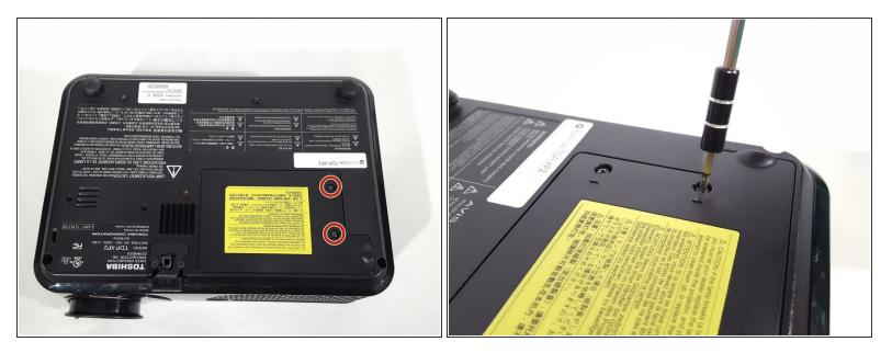
• Remove the two screws from the bottom plate as shown.
