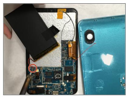
Make contact with the battery terminals with the hot tip of the soldering iron for a few seconds while slowly pulling the wire away.
