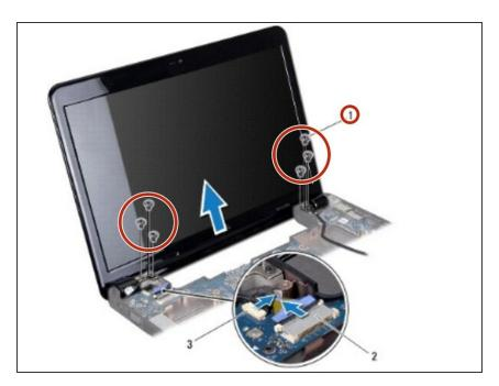
Place the **NEW** display assembly in position and replace the six screws (three on each side) of the display assembly.
