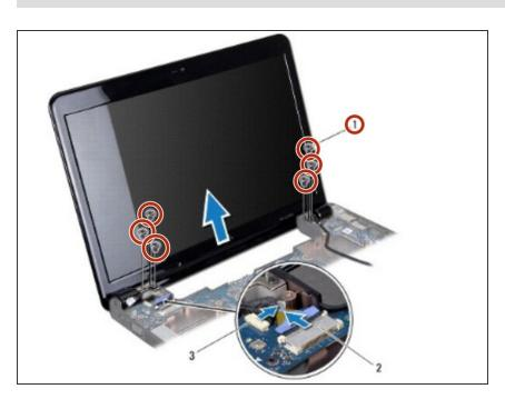
Remove the six screws (three on each side) that secure the display assembly to the computer base.
