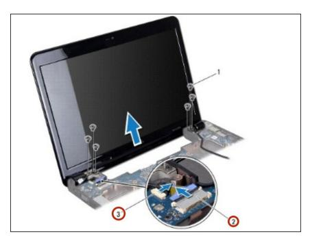
Connect the display cable and the camera cable to their respective system board connectors.
