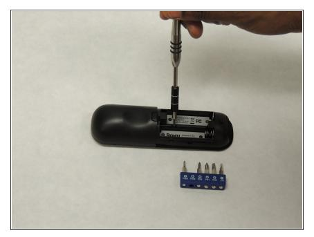
Remove the screw using a Phillips #00 screwdriver.
