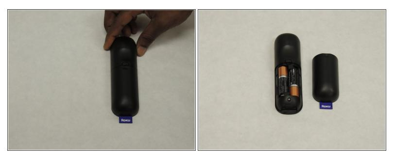
• Flip the remote so that the buttons lay face down and then remove the back cover.
