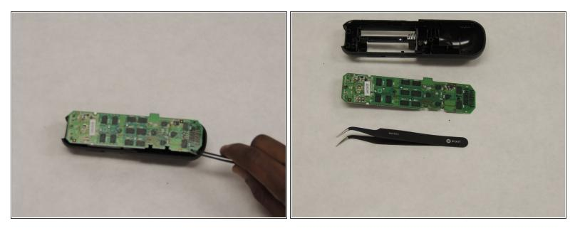
• Using tweezers, remove the motherboard from the remote.
