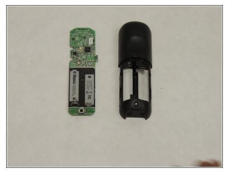
• The contacts should be present with one set being in the bottom of the remote casing and the other set being on the underside of the motherboard for the remote.
