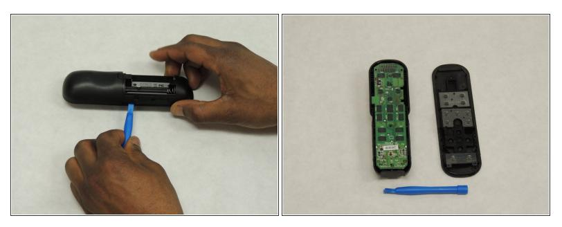
• Remove the face of the remote with the plastic opening tool.
