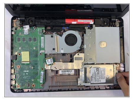
Remove the hard drive by pulling it towards the right, and removing it from the laptop case
