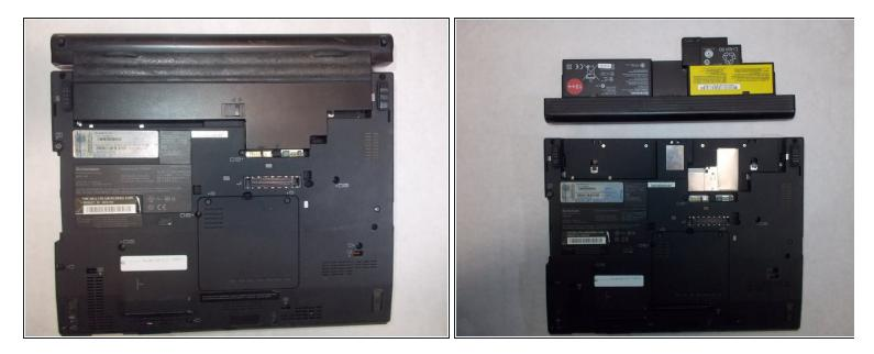
• Slide out the battery near the top of the laptop.
