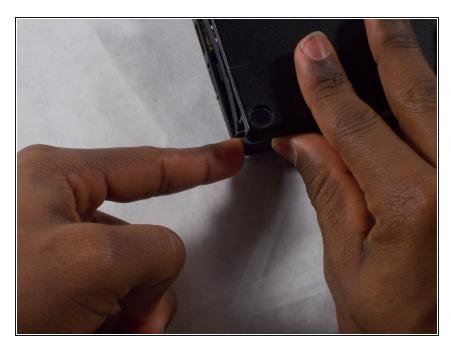
• If step 4 does not work, gently push the bar down while using your other hand to pull the trackpad up.
