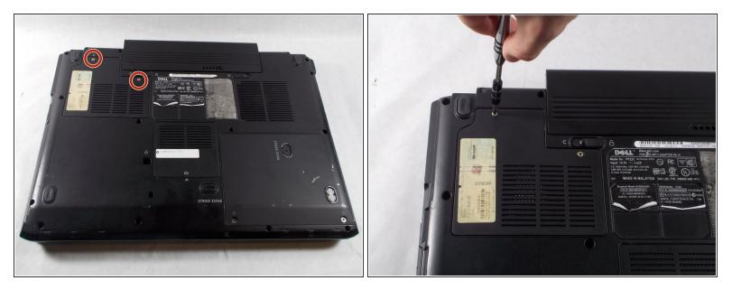
• Remove the two Phillips #1 screws from the Wi-Fi card cover on the bottom of the laptop.
