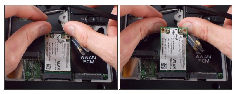
• Use your thumbs to push the retaining clips upward to release the card.
