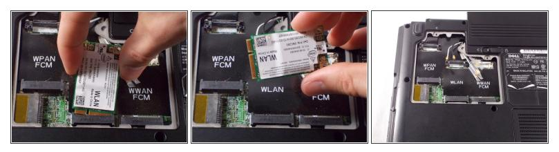
• Pull the card outward and then upward to remove it from the slot.
