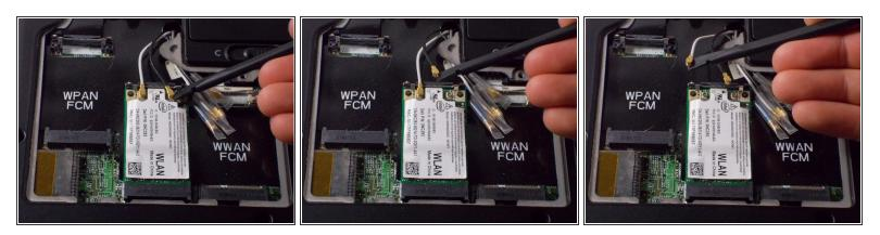
• Use the spudger to lift the small wires connecting to the Wi-Fi card.
