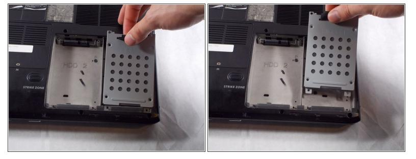
• Lift and remove the Hard Drive and chassis out of its the slot.
