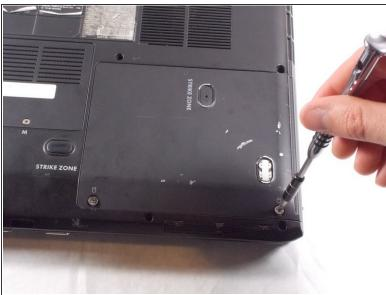
Remove the two 4.5mm Phillips #1 Screws that hold the HDD cover in place.
