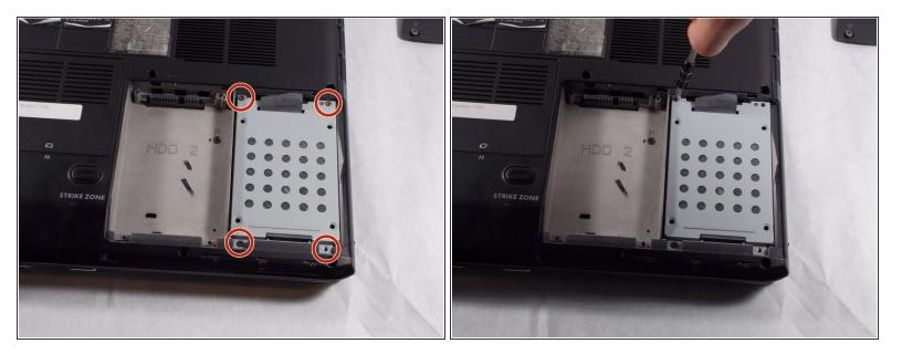
Remove the 4 Phillips #0 screws that hold the HDD chassis in place.
