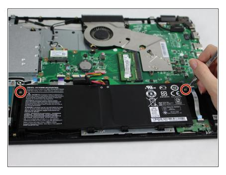
Remove the two 5 mm screws located on either side of the battery.
