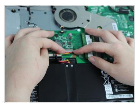
Disconnect the colored bundled cable connectors from the motherboard. To do this, pull on the wires to disconnect the cable and remove the battery.
