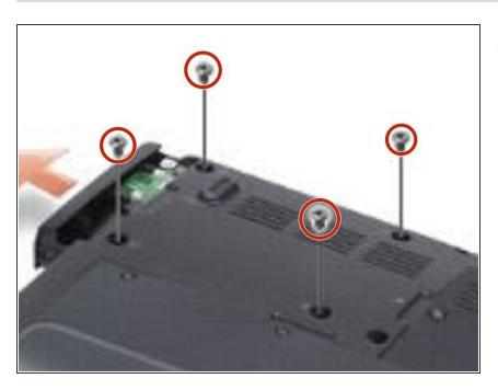
Replace the four M3 x 3-mm screws on the hard drive.
