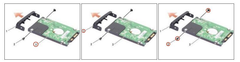
● Place the **NEW** hard drive in the bracket and replace the two M2 x 3-mm screws on either side.
