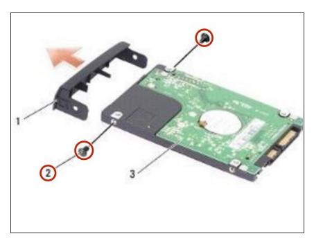
Remove the two screws from either side of the hard drive bracket and pull the hard drive away from the bracket.
