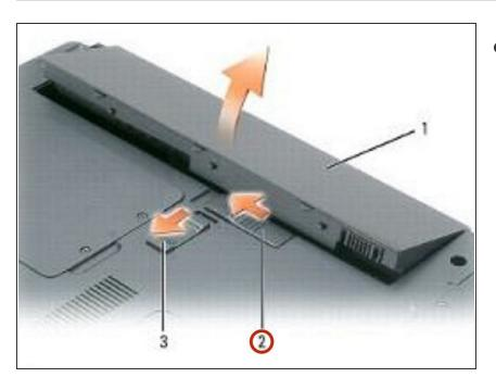
Slide and hold the battery-bay latch release, and then remove the battery from the bay.
