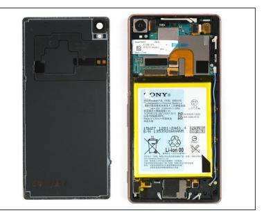
After pulling out the adhesive tabs, you can lift the back cover and remove it.
