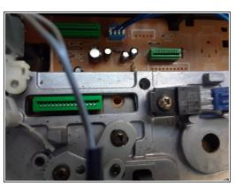
before removing the plate disconnect these three wires to preserve the functions of the VCR.
