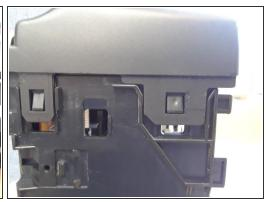
After removing the cover you must unclip all the clips of the front paneling
