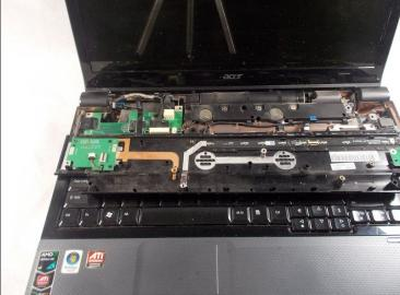
• Lift the top panel up from the back, turning it over forward.
