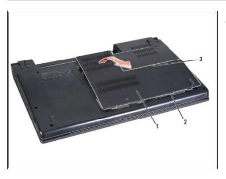
Loosen the three captive screws on the base cover and lift the base cover off the computer at an angle as shown in the figure.
