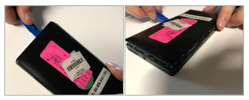
• Wedge a plastic opening tool between the two panels. Slide it along each side of the phone to completely remove the back panel.
