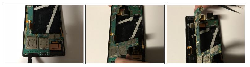
• Use a spudger to pry up the bottom end of the motherboard, then pull it out.
