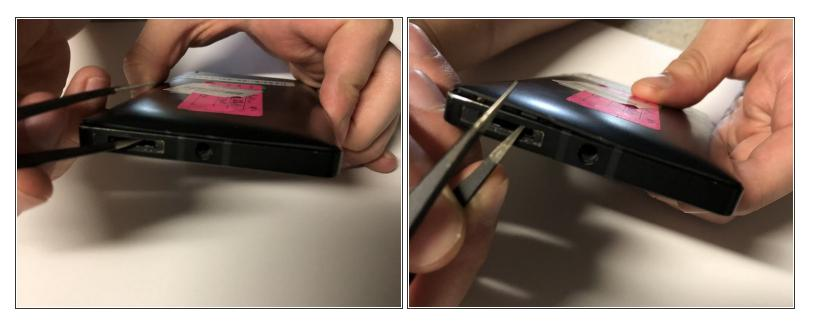
Place tweezers or an opening tool in the SIM card slot and push upwards until the back panel pops out.
