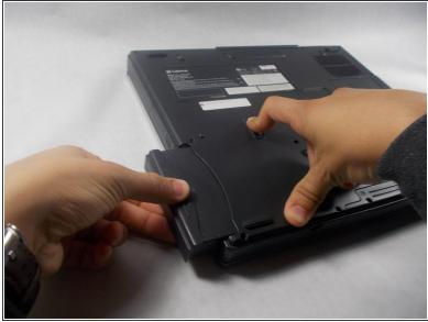
• The next step is to simultaneously push up on the battery release button and to pull out on the battery itself. If this is not done simultaneously then the battery will not budge.
