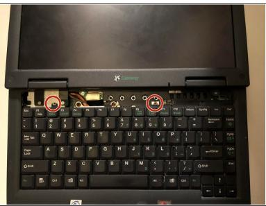
The two J0 screws have now become visible. Using the Phillips J0 screwdriver, remove screws.
