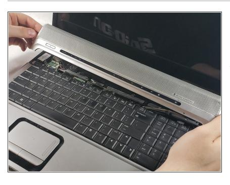
With the ribbon cable successfully detached you may now replace the media bar with a new, functioning one.
