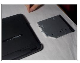
Remove the disk tray assembly by sliding it out from the side using the blue plastic opening tool.
