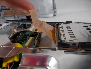
Pull the ribbon tab up and off the motherboard.
