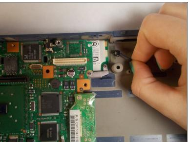
Pinch your fingers around the base of the connector and pull it out.
