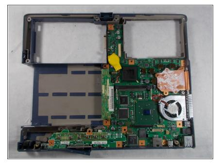
Remove the metal plate covering the motherboard.
