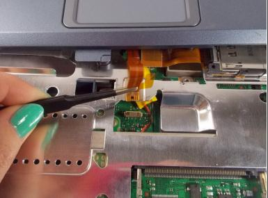
Remove the ribbon from the motherboard with a pair of tweezers.
