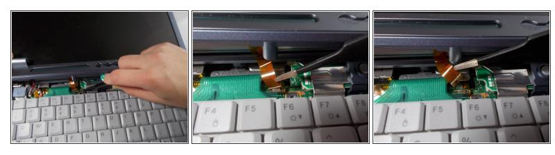
Use the tweezers to disconnect the ribbon cable from the motherboard.
