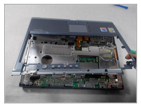
Lift up the plastic frame from the base to expose the ribbon attached to the motherboard.
