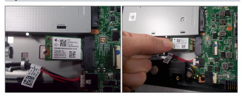
• Pull up on the wireless card and remove it from the device.
