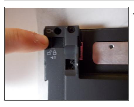
The next step is to simply move the switch from the locked position to the unlocked position.
