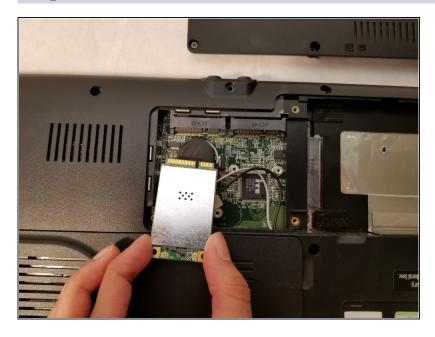
Lift and pull the Wireless LAN card away from the computer.
