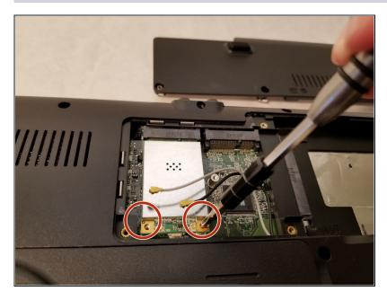
Using the Phillips #1 screwdriver, remove the two 2.5mm screws holding down the card.
