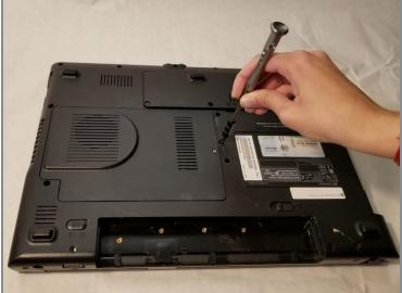
Using the Phillips #1 screwdriver, remove the four 6mm screws on the back of the laptop.
