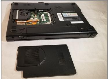
• Insert the plastic prying tool and pry the back panel off starting at an edge and moving your way around it.
