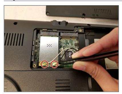
Use the <u>tweezers</u> to remove the two connecting wires.
