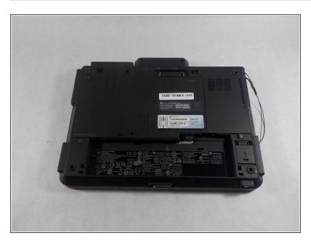
Lift and remove the battery from the battery compartment.
