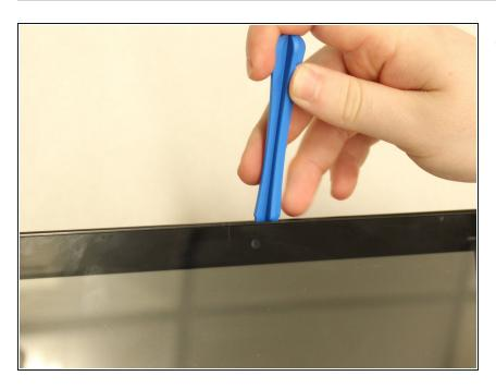
• Use the plastic opening tool to separate the screen from the back cover.
