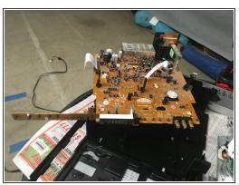
Now, you will remove the large, orange motherboard. You will need to unscrew it and pop it out. You MUST be careful as this piece is extremely fragile, and the smallest fracture or damage will cause it to no longer work.
