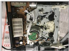
Now you can unscrew the VHS receptor and remove that to be able to access, unscrew and remove the final piece, the large motherboard.
