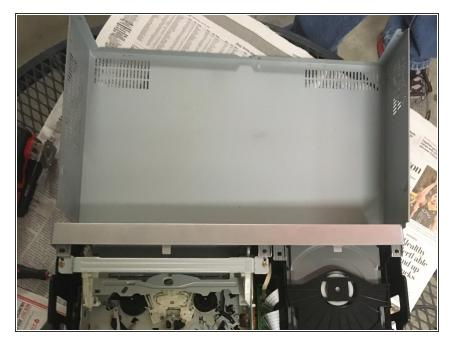
Now, you need to remove the cover by lifting it up like you would the cover of a shoe box, but it will come off. But before you do that you will need to unhook it by unclipping the clips on the back.
