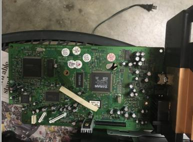
Now that the DVD tray is out of the way, you can remove the smaller motherboard, the green one to specify easier. You will do this by removing the screws that hold it in.
