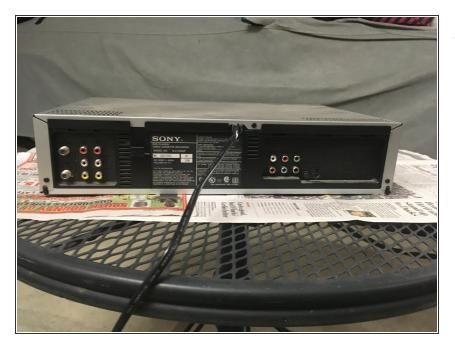
First, you need to remove the three black screws on the back.
