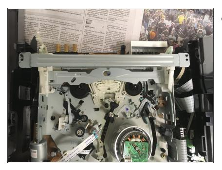
You must now remove the silver bar attached to the VHS receptor.
