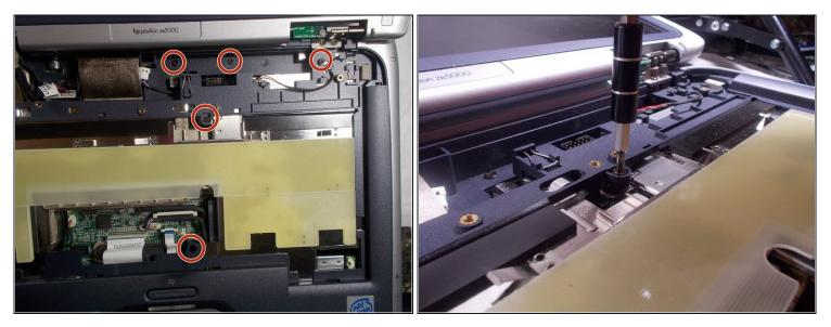
• Remove the five 5.0 mm Phillips #1 screws from underneath the keyboard
