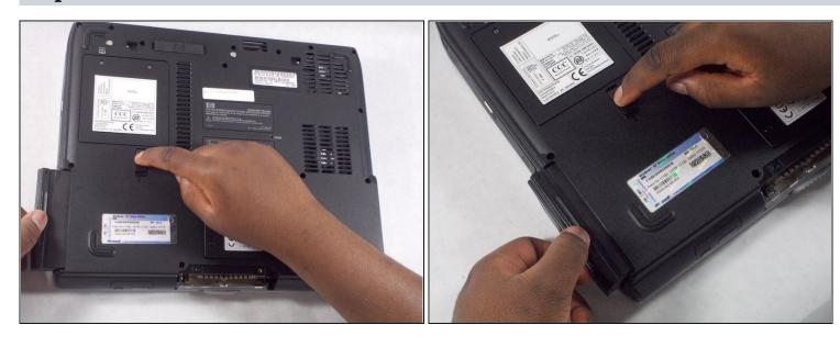
• While still holding the switch up, remove the battery.
