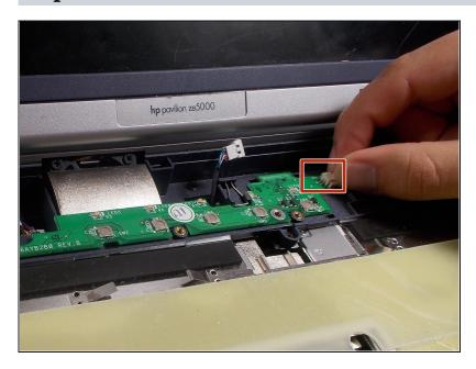
Gently remove the disconnection to the right of the circuit board
