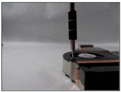
• Remove the eight 3.5 mm Phillips #00 screws from the fan housing unit
