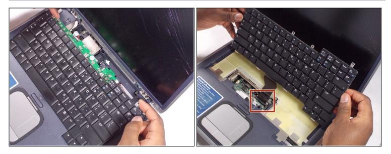
• Gently lift the keyboard up from the frame so that you can see the ribbon still connected.
