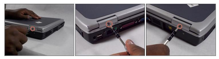
• Remove the two 5mm Phillips #0 screws from the hinges
