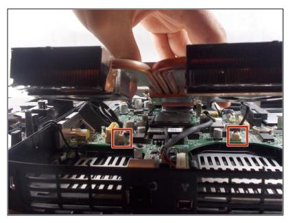
Lift the housing unit a few inches from the device to expose the two small connections.
