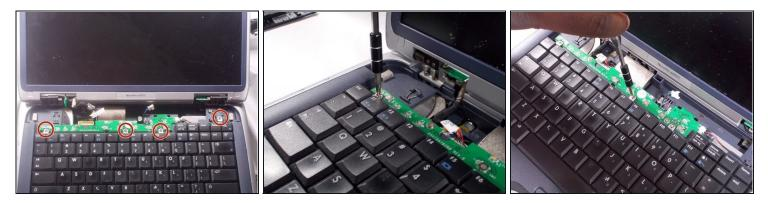
• Remove the four 4.0 mm Phillips #0 connecting the keyboard to the frame
