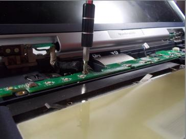
Remove the two 4.0 mm Phillips #0 screws attached to the cicuit board above the keyboard
