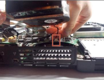
• Remove the two small connections directly above and below the fan housing unit
