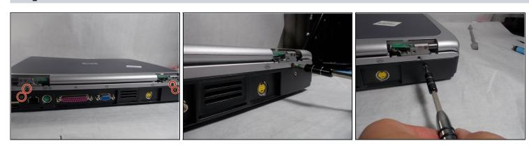
• Remove the additional four 5.0 mm Phillips #1 screws from the hinge of the device
