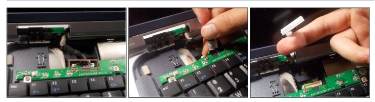
Remove the connection beneath the left hinge of the device
