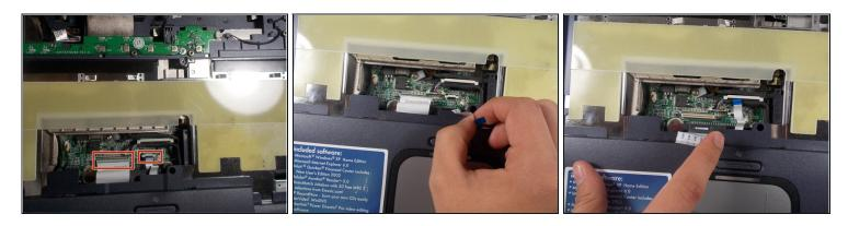
Disconnect the ribbons from the circuit board underneath the keyboard housing unit
