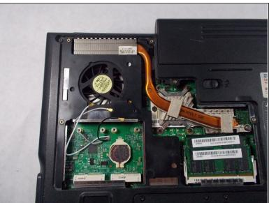
With the WiFi Card lifted up, gently pull the WiFi Card out of the socket and remove it from the device.
