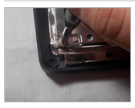
At each corner, there is a 1 centimeter silver screw connecting the screen frame to the laptop.
