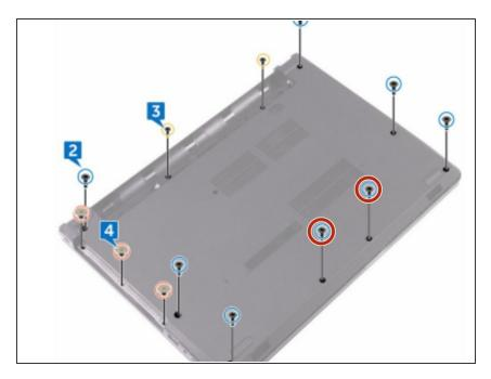
Remove the two screws that secure the base cover to the palm-rest assembly.
