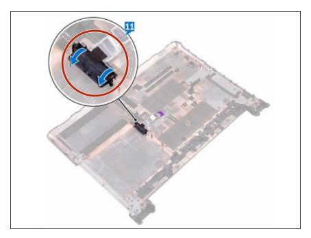
Release the optical-drive interposer from the tabs, and remove it from the base cover.
