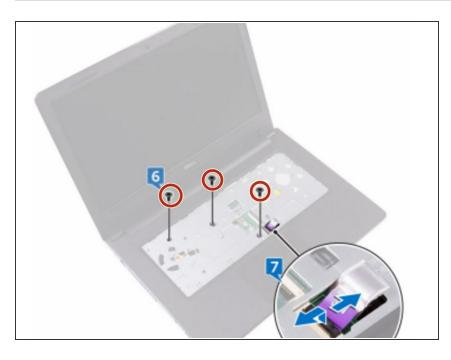
Replace the three screws (M2x5) that secure the base cover to the palm-rest assembly.
