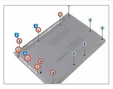
Remove the eight screws that secure the base cover to the palmrest assembly.
