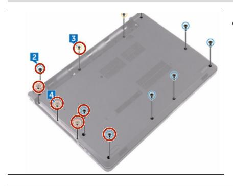
Replace the eight screws that secure the base cover to the palmrest assembly.
