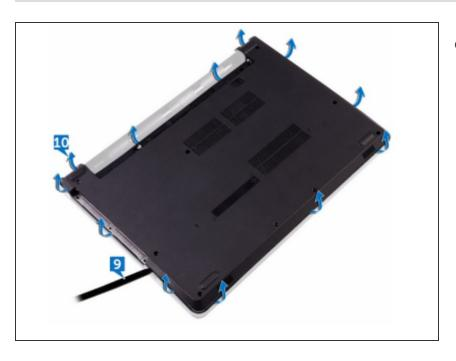
Lift the base cover off the palm-rest assembly.
