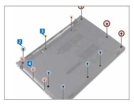
Remove the three screws that secure the base cover to the palmrest assembly.
