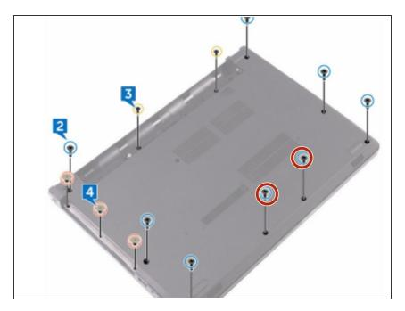
Replace the two screws (M2x5) that secure the base cover to the palmrest assembly.
