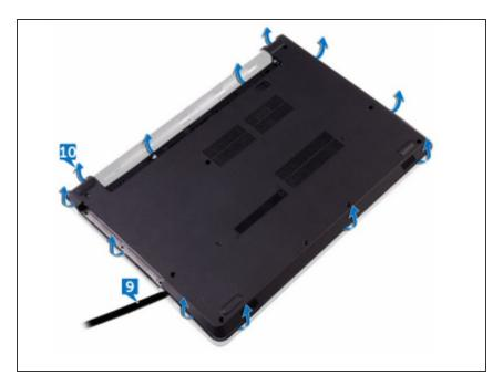
Using a plastic scribe, pry the base cover off the palm-rest assembly.
