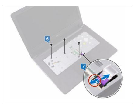
Open the latch, and disconnect the optical-drive cable from the system board.
