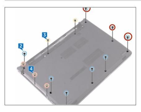
Replace the three screws (M2x2) that secure the base cover to the palm-rest assembly.
