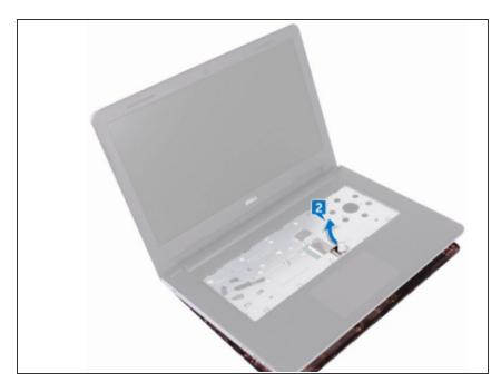
Slide the tabs on the base cover into the slots on the palm-rest assembly, and snap the base cover into place.
