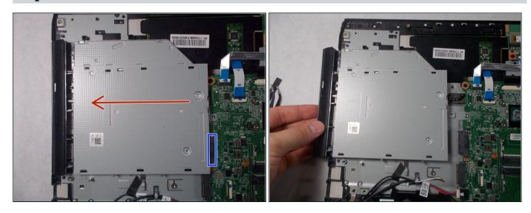
• Gently pull the CD drive out, disconnecting it from the motherboard connector marked in blue.
